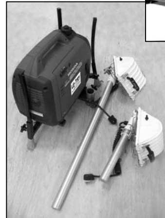
Figure 8: Dual unit with lights disconnected
